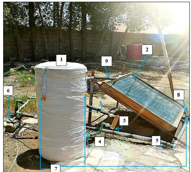
Fig. 1 Photograph view of solar water heater 1. Storage tank. 2. Solar collector. 3. Flowmeter. 4. Valve. 5. Insulation pipes. 6. Pump. 7. K-type thermocouple of the inlet, outlet, and storage tank, 8. Collector inlet, and 9. Collector outlet.
